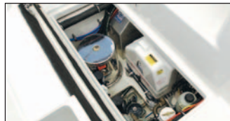
4.2 KW DIESEL GENERATOR W/12 GALLON TANK R305
